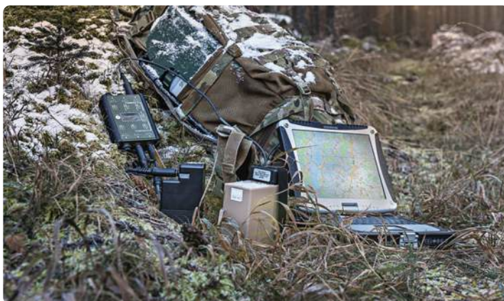
SFC JENNY fuel cells supply electrical devices in the network
